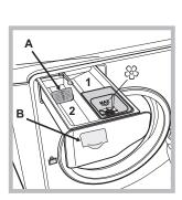
The detergent dispenser drawer is located inside the machine and can be accessed by opening the door.
